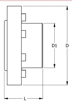
D = 200 D1 = 140 L = 90 Max bore = 85 Torque (N m) = 1340
